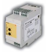
Measuring the regenerated voltage on a motor's coils, is the best way to determine if the tool on a motor's shaft is moving. This operation must be performed safely in order to comply with safety category 3. The MF1C provides this function, allowing for the opening of the lock of a safety gate only when the motion of a motor has come to a complete stop.
